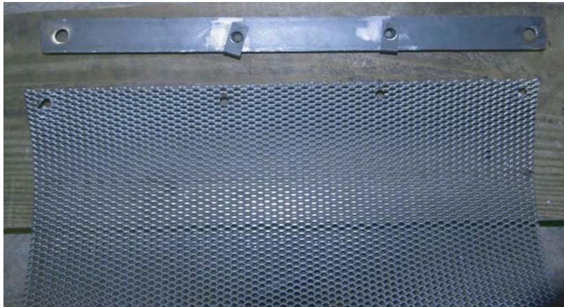
This serves two purposes: 1. It keeps the hole in the screen the same size (1/4") as the supplied bolt shank to just pass through so there is no slop under head, to keep from weakening the screen.
