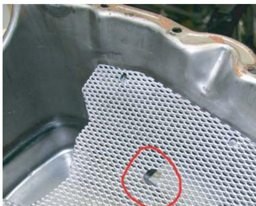
12. Make sure to clean the pan and windage screen related parts extremely well of all metal dust, shavings, etc. and reinstall the screen into the pan, then the pan to the motor (with gasket this time). At this point you are done and you have just installed a windage screen in your oil pan for better oil control!
