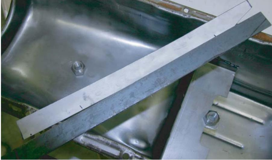
I started on the passenger side rail and trimmed it to length. I then clamped the screen on top of the rail, leaving about 1/16" of the rail sticking above the screen to leave room to weld to the pan side
