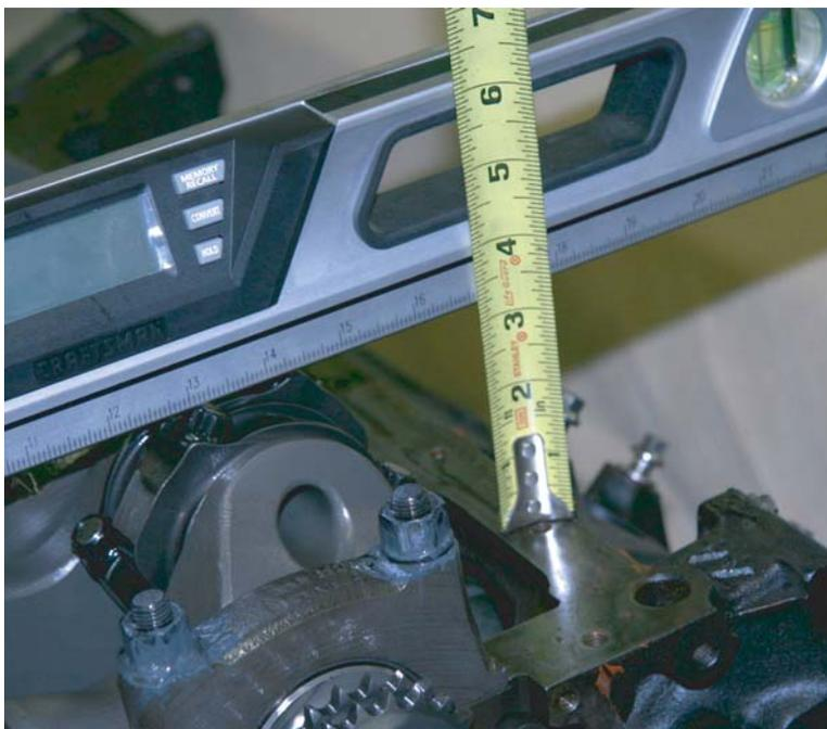
2. Using the oil pan bolt on both sides nearest the 1 / 2 rod combo as reference, measure in the same spot from the oil pan rail to the floor of the pan, again with a straight edge across the pan rails. Record this measurement on paper.
